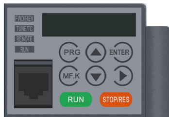
Figure 4-1 Diagram of the operating panel
