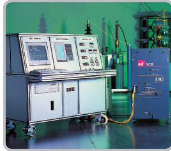
Characteristics Test / VCB Characteristics Test
