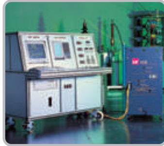
Characteristics Test / VCB Characteristics Test
