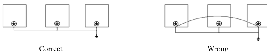
Figure 3-8 Grounding Wire Connection Sketch Map
