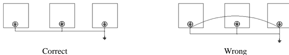
Figure 3-8 Grounding Wire Connection Sketch Map
