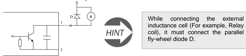
Fig.6-12 Inner wiring diagram of output terminals
