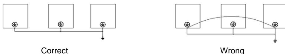
Figure 3-6 Connection of conduction and radiation interference solutions
