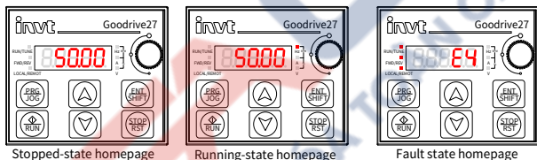
Figure 5-2 Status interface display
