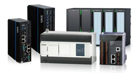
XS series PLCopen standard controller, developed based on CODESYS platform, has two platform architectures of X86 and ARM, which can meet users requirements for high-speed and low-speed computing in various occasions.
