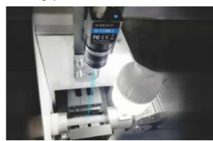
In view of the problems that the traditional pipe cutting scheme cannot accurately cut the deformed hose, X-SIGHT launched the hose positioning and deviation correction cutting system, which automatically compensates the cutting point offset to ensure the accuracy of knife dropping, with an accuracy of up to 0.05mm.
