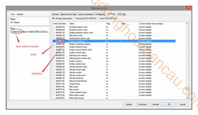
The figure shows the slave and the corresponding object dictionary index, read the value in slave object dictionary 0x6060: 00 of StationID0 to D0.
