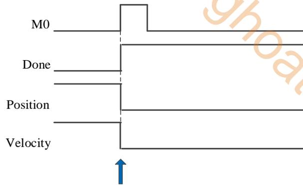
The position when triggered is the position where the axis stops
