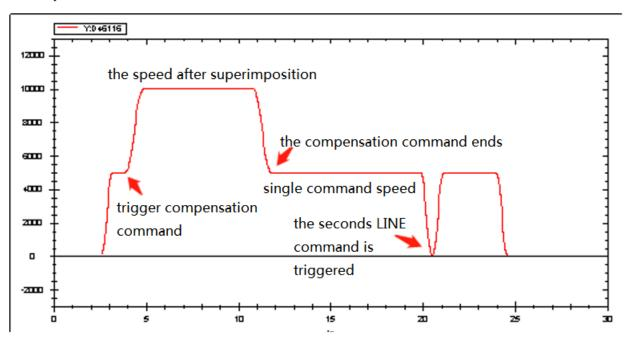
It can be seen from the position curve that after the execution of the first instruction and the superimposed instruction, the position is 70000 (including the compensation value of the superimposed instruction to the position of 20000), and after the execution of the second line instruction, the final position is 80000 (the instruction parameter is 60000), so it can be seen that the compensation of the compensation instruction to the position is always effective.
