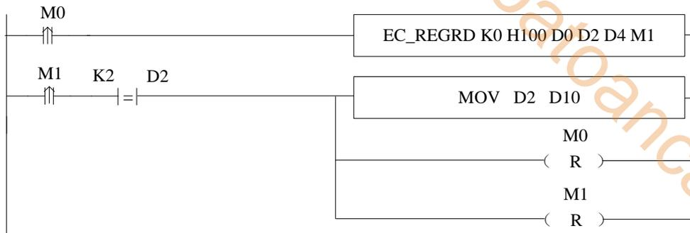
After operand S5 (M1) is set ON, check the status of S4 (D2). According to the status code, if the instruction is processed successfully, the read register can be set value. Since the completion mark M1 will not reset actively, it needs to be reset manually, so RST M1.
