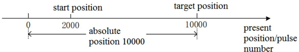
The target position in the command is the absolute position from zero point to target point, so moving to the position of 10000 pulses requires setting the target position 10000. Similarly, moving to the position of 20000 pulses requires setting the target position 20000.
