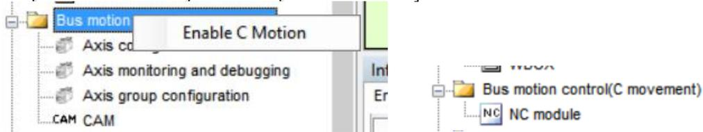
When selecting H motion, the project bar shows [axis configuration], [axis monitoring and debugging], [axis group configuration]. When selecting C motion, it shows [NC module].
