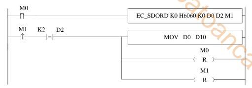
After operand S5 (M1) is set ON, check the status of S4 (D2). According to the status code, if the instruction is processed successfully, the read register can be set value. Since the completion mark M1 will not reset actively, it needs to be reset manually, so RST M1.
