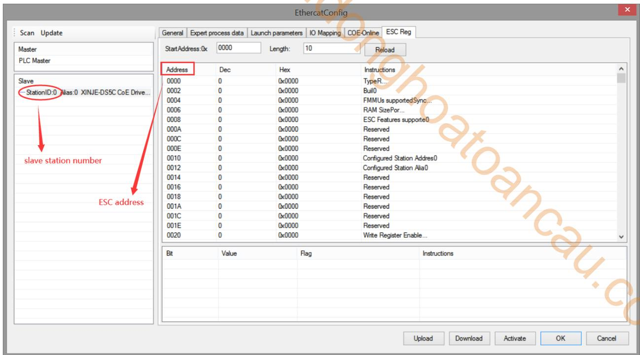
The figure is ESC parameter interface, if it needs to read ESC address H100 of slave station StationID0, please see below example.
