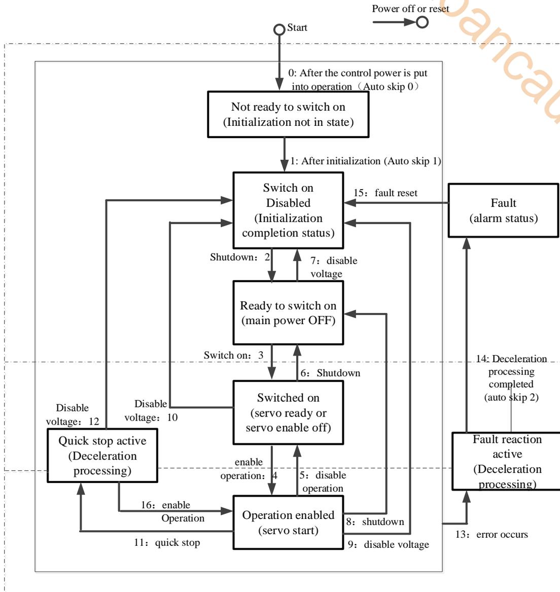
After migrating to operation enabled(servo is enabled), please increase the time to more than 100ms and input the action command.
