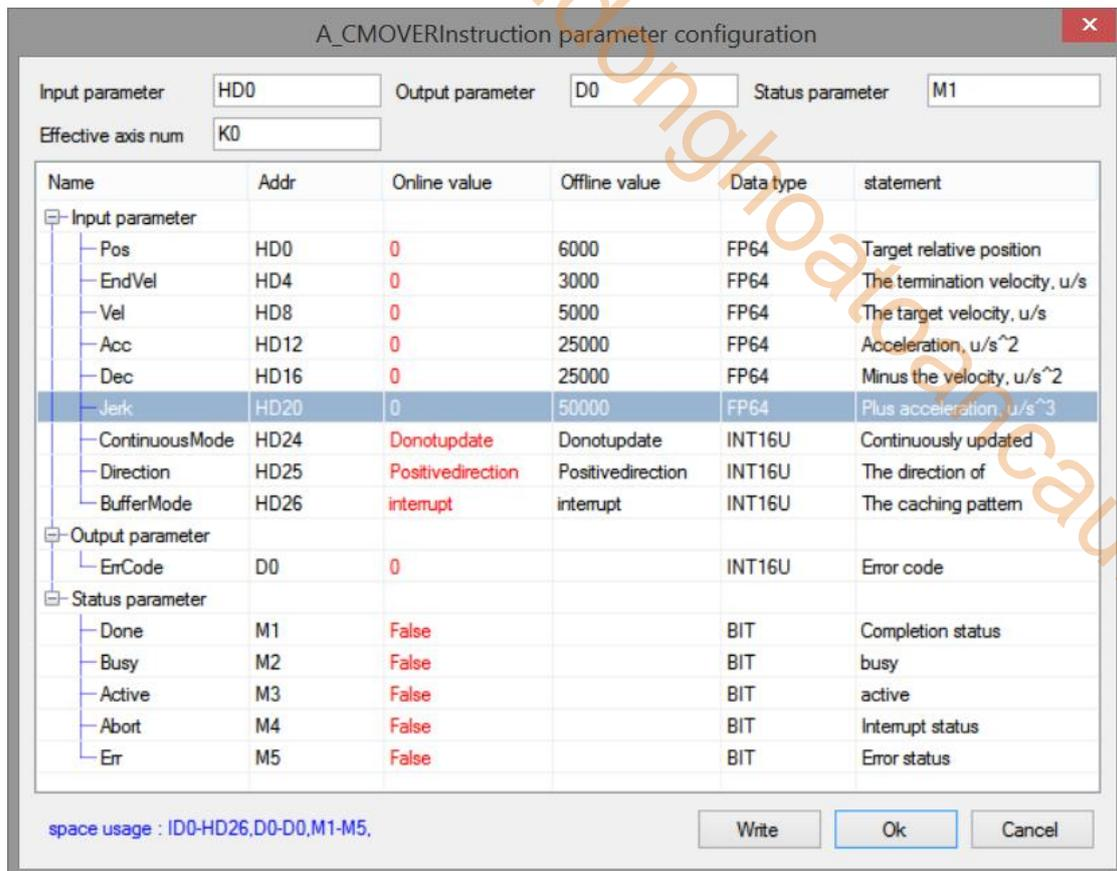
Note: to enable the axis with A\_PWR instruction. After confirming that the enabling is successful, M0 is turned from off → on to trigger A\_CMOVER command, the command runs to the target relative position at the set speed, and then runs continuously at the termination speed. During operation, the state machine D20000+200\*N of the axis is 3.
