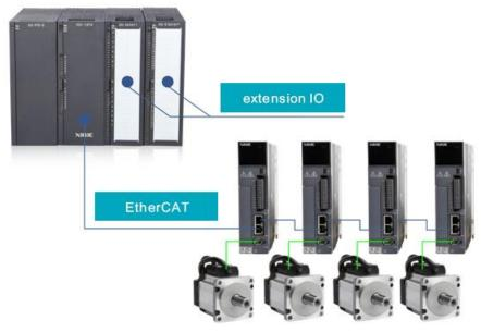
Note: only LIN2 port in XG2 series PLC supports EtherCAT communication. The two communication network ports of the servo driver follow the principle of "down in and up out", that is, the link2 port of XG2 must be connected with the network port under the LIN1 port of the first servo, and then the network port above the first servo is connected with the network port under the second servo, and so on.
