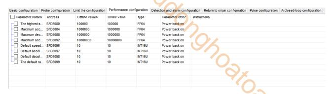
As the above figure, the default speed=100000 (max speed) \*10% (default speed percentage) =10000. If the maximum speed of the single axis is set low, the axis group will calculate the linear speed according to the maximum speed of the single axis, so that the linear speed of the axis group cannot reach the target speed set in the command.
