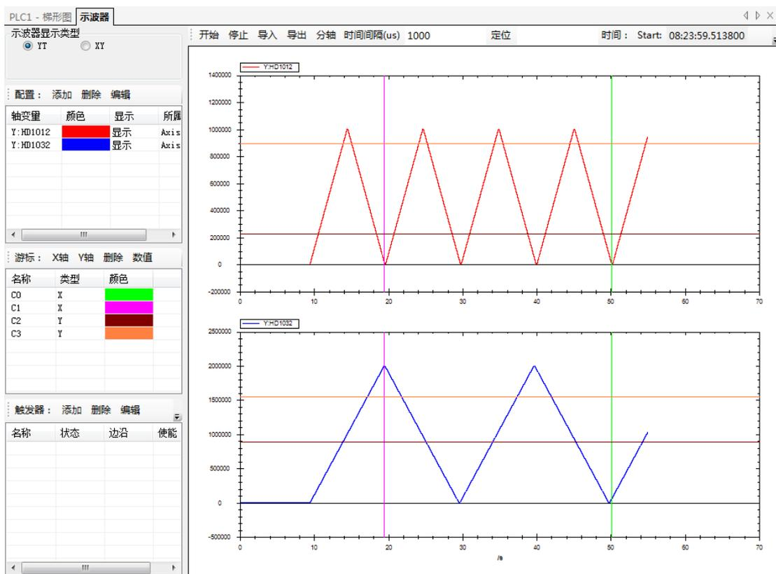
Click the cursor configuration [value] to enter the cursor difference interface, which can monitor the specific value of the register with the cursor.
