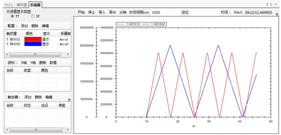
There are two coordinate axes on the left, axis 2 ordinate on the left and axis 1 ordinate on the right.
