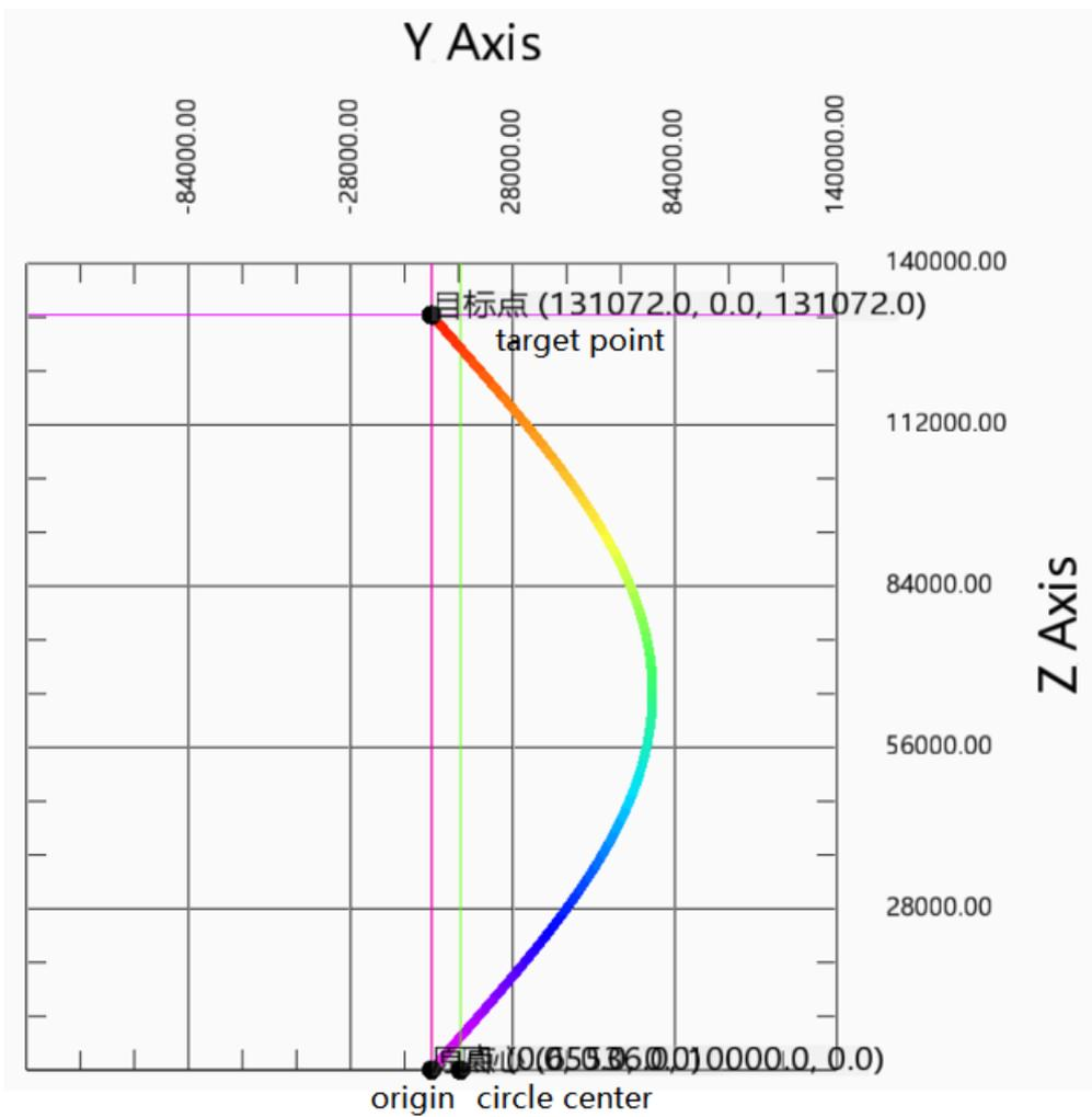
Action decomposition: the two axes of XOY plane do plane arc action, and the arc track is determined by the starting point, center, target coordinates and path selection on the selected plane. The Z-axis moves in a straight line at a uniform speed, and the moving distance is the difference between the starting point of the Z-axis and the target point. The three axes start and stop at the same time, and the three-axis speed is decomposed into XOY plane linear speed and Z-axis linear speed.
