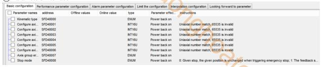
[Basic configuration]: corresponds to the register SFD48000+300\*N~SFD48008+300\*N, refer to chapter 5-2-3. [Performance parameter configuration]: corresponds to the register SFD48020+300\*N~SFD48059+300\*N, refer to chapter 5-2-3.
