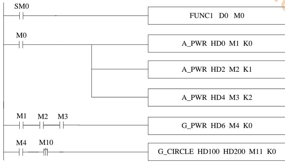
Among them, FUNC1 function block is used to set value for G\_CIRCLE command, M0 turns on the enabling of each axis. When all three axes enabling are turned on (flag bits M1, M2 and M3 are on), turn on the axis group enabling. After the axis group is enabled (the flag M4 is on), when M10 is set to on, execute the G\_CIRCLE command.
