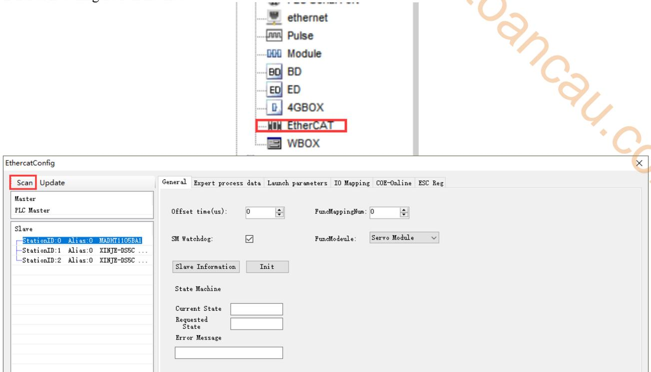
② confirm the PDO in the [expert process data] (The default configuration can meet the use of instructions. If necessary, other relevant parameters can be added).
