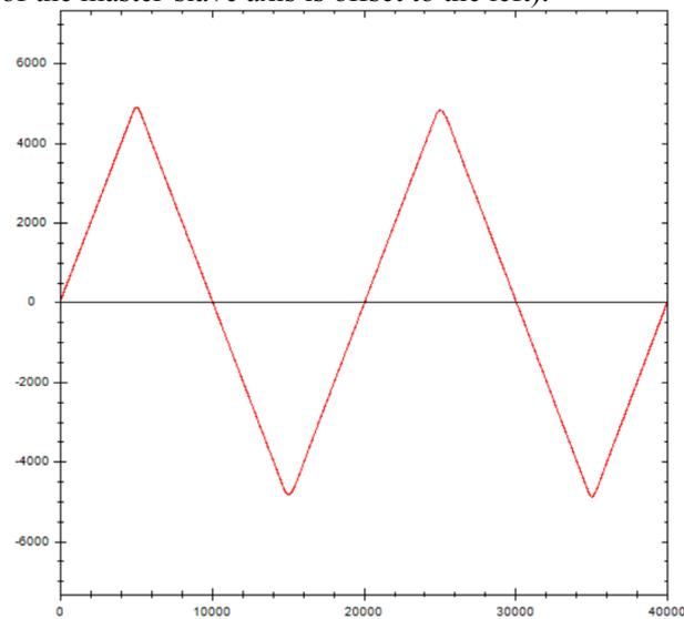
When the ratio of the master and slave axis is 1 and the offset of the slave axis is 5000 (the offset of the slave axis is valid only when the slave axis is in absolute or tracking mode, which will step/catch-up to the offset position when the CAMIN command is triggered, and the alarm of the slave axis may be caused in absolute mode):
