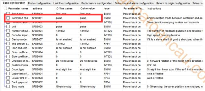
(2) Set the pulse port and pulse direction port in axis configuration-probe configuration. Pulse port range is [0,3], direction port range is [0,7],[10,17],[20,27].
