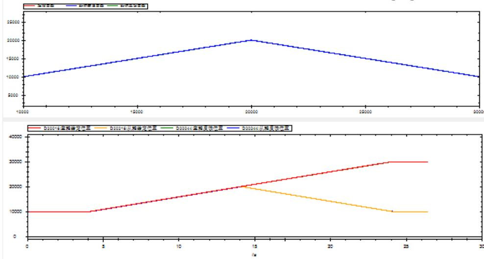
It can be seen that the starting point of the track is (10000,10000), and the entire cam table is executed.
