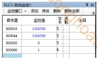
The given position (D20016) and the current position (D20044) are the final position 1310720 set in the command, the current given speed (D20020) is 0, and the current axis state (D20000) is 1, indicating that the axis is in the enabled static state.
