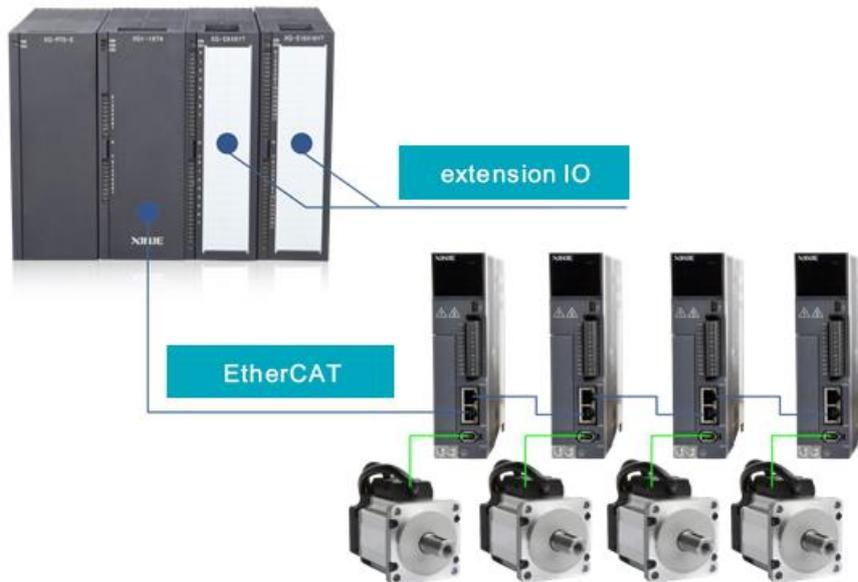
Note: only LIN2 port in XG2 series PLC supports EtherCAT communication. The two communication network ports of the servo driver follow the principle of "down in and up out", that is, the link2 port of XG2 must be connected with the network port under the LIN1 port of the first servo, and then the network port above the first servo is connected with the network port under the second servo, and so on.
