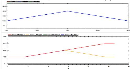
It can be seen that the starting point of the track is (10000,10000), and the entire cam table is executed. When the main axis adopts relative mode and the slave axis adopts absolute mode, and the starting position of the master and slave axis is 10000, the track of the executed cam table is shown in the following figure
