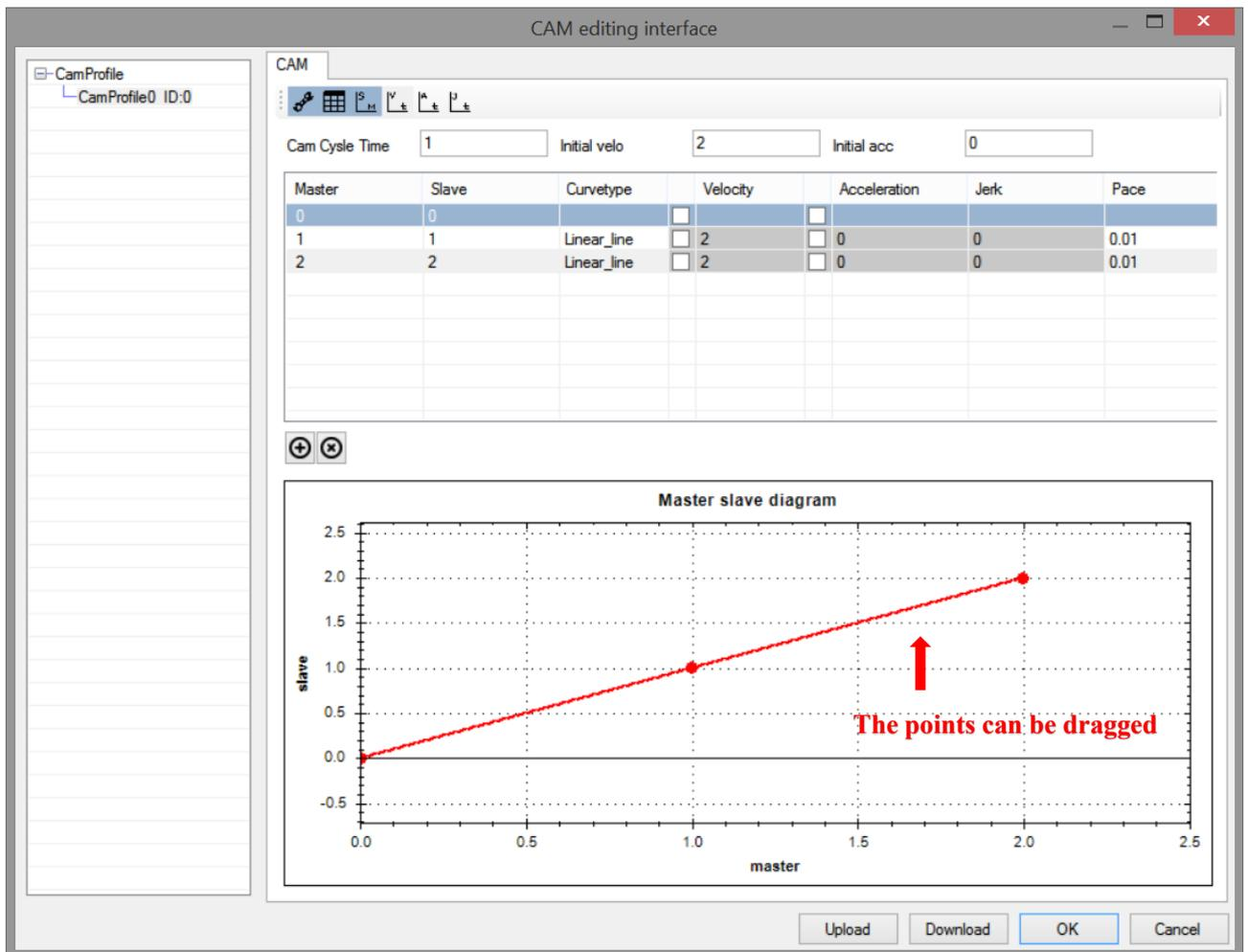
[main axis]: The point position of the main axis can be changed manually by double clicking. The subsequent point position must be greater than the previous point position. The number of main axis points cannot exceed 65535. The number of main axis points = (main axis final point position – main axis starting point position) / pace
