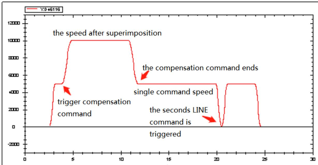
It can be seen from the position curve that after the execution of the first instruction and the superimposed instruction, the position is 70000 (including the compensation value of the superimposed instruction to the position of 20000), and after the execution of the second line instruction, the final position is 80000 (the instruction parameter is 60000), so it can be seen that the compensation of the compensation instruction to the position is always effective.
