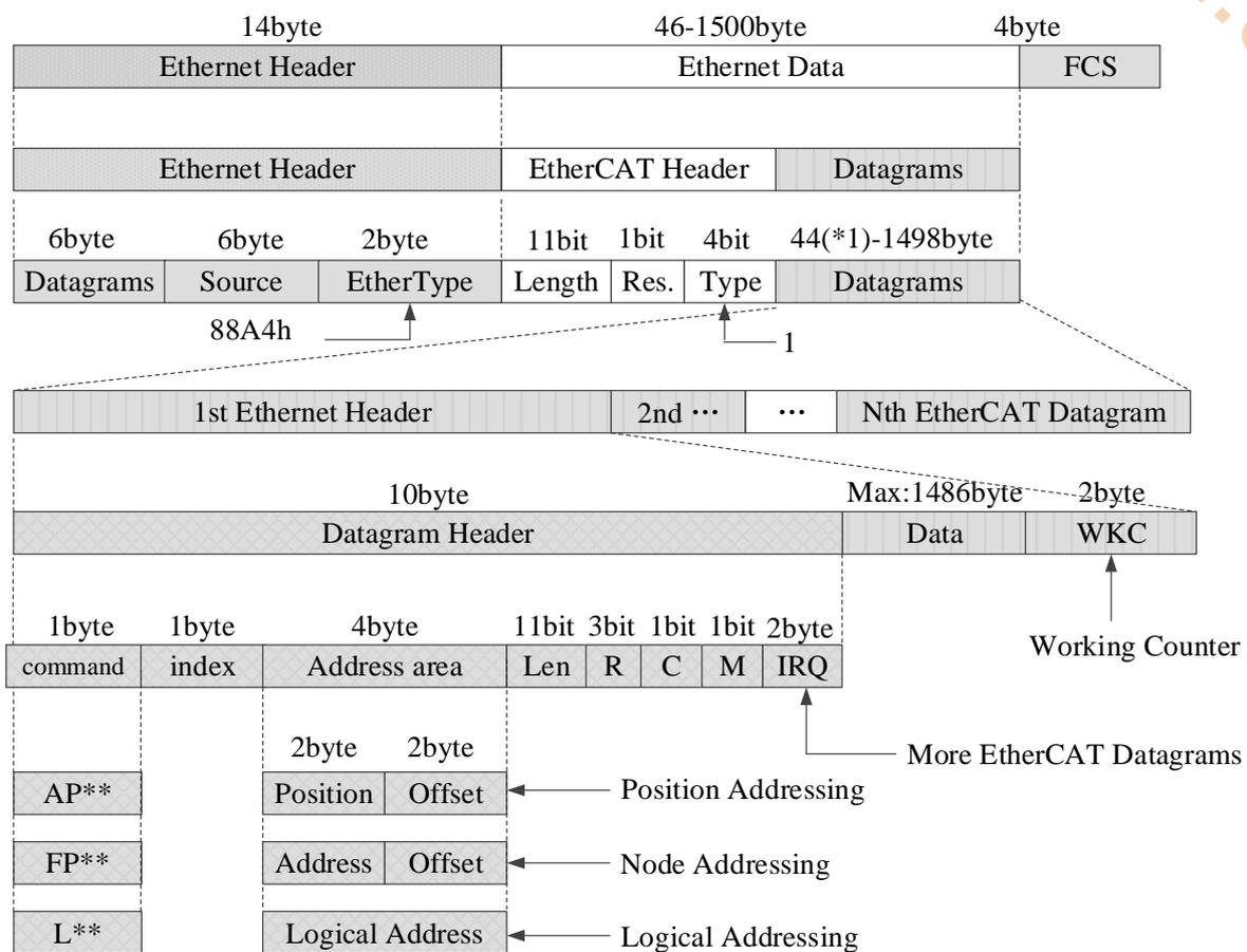
\*1: Ethernet frame is shorter than 64 byte, 1-32 byte is added.
