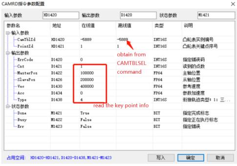
The cam table instance number is obtained through CAMTBLSEL command. The key point sequence number should start from 0, and 0 represents the first point (0,0) of the cam table.
