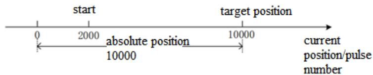
The target position in the command is the absolute position from zero point to target point, so moving to the position of 10000 pulses requires setting the target position 10000.
