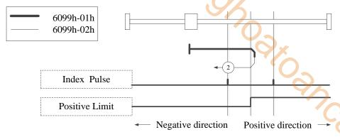
Homing on positive limit switch and index pulse
