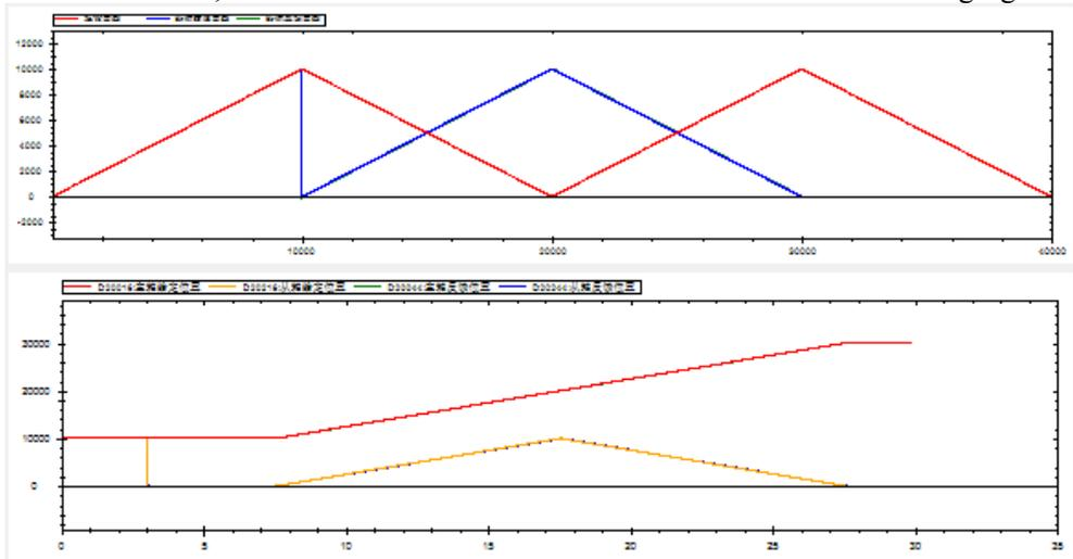
It can be seen that the starting point of the track is (10000,0), and the entire cam table is executed, and the slave axis position produces a step from 10000 to 0 at the beginning.
