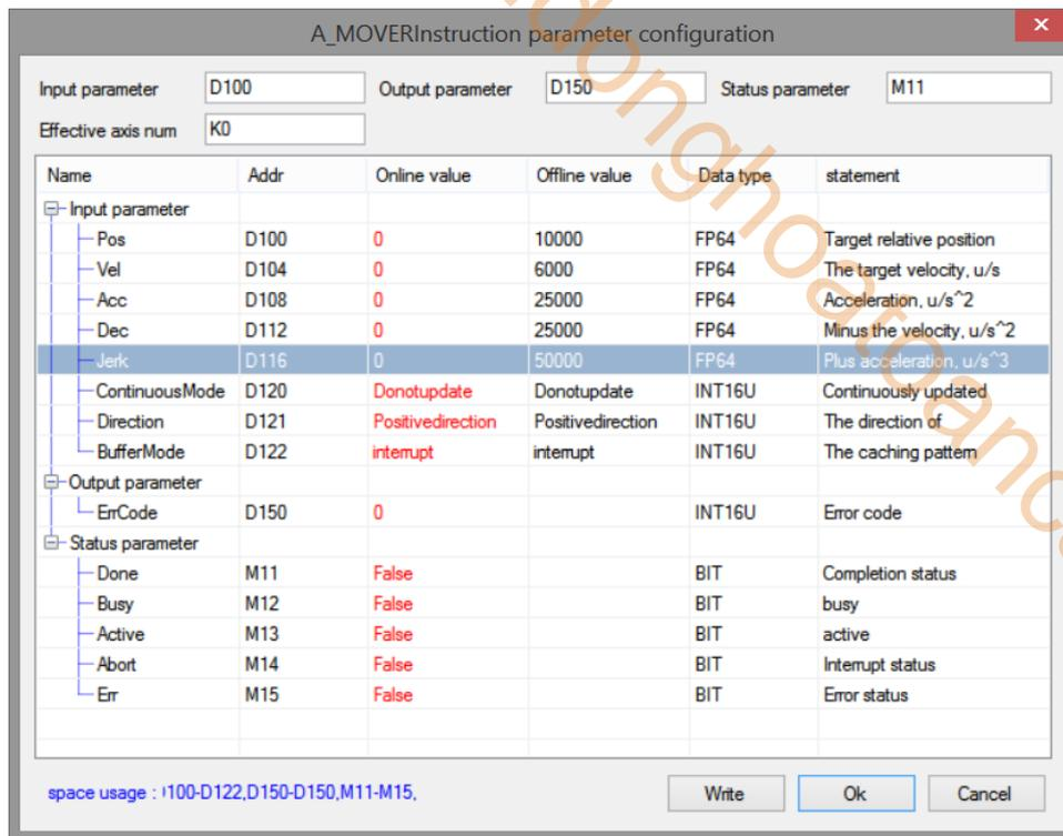
Note: first turn on the enable through A\_PWR command. When M2 is turned from off to on, it runs to target position 1 with the parameters set in the first command. After reaching the target position, the state parameter M3 of the command is turned from off to on, so the second A\_MOVER is triggered, and finally run to target position 2 with the parameters set in the second command.
