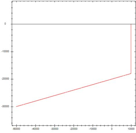
In the figure, the abscissa is X axis and the ordinate is Y axis. Coordinate starting point (- 50000, - 30000), after G PTP motion, the X and Y axes move to the target position (10000,0) at their respective default speeds.
