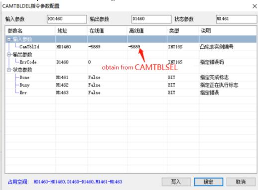
The cam table instance number is generated by the CANTBLSEL command. After the command is executed, the instance will be unloaded. If the instance number has been started by the CAMIN command, you need to execute the CAMOUT command to release the cam relationship, and then execute the unloading command.
