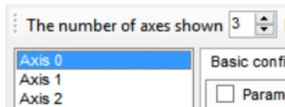
The setting of [the number of axes shown] determines the number of axes in the configuration bar. It has nothing to do with the actual number of connected axes and is only for display. Select the corresponding axis number to configure the axis related parameters.
