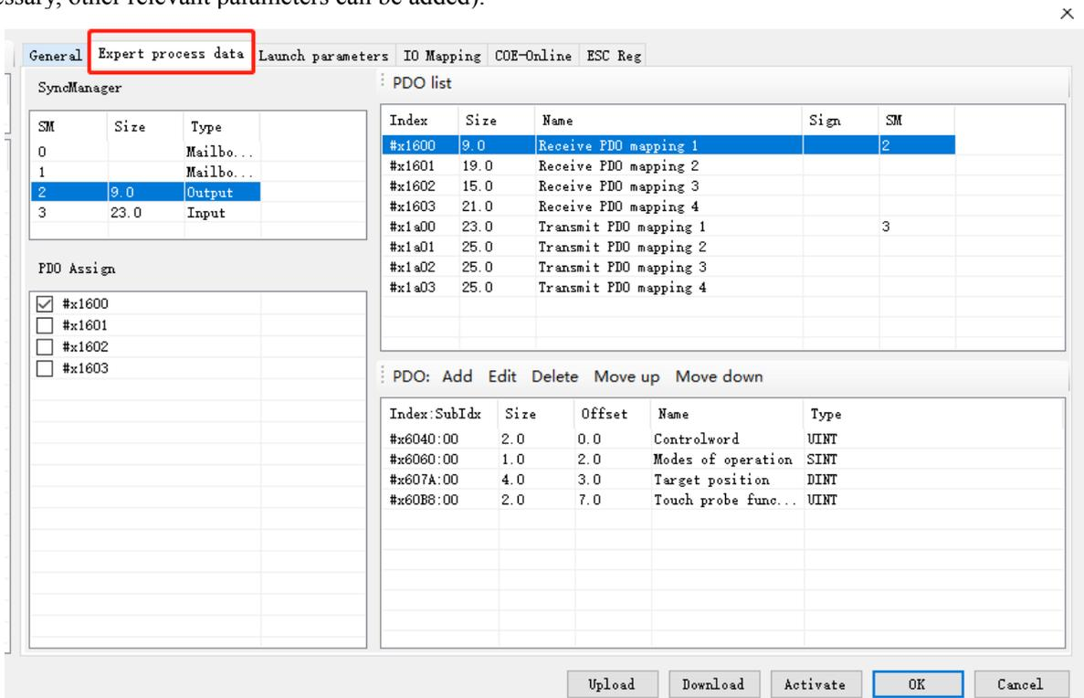
③ confirm the value of 6060h is 8 in [launch parameters]. 6060h value 8 represents the slave station is CSP mode.
