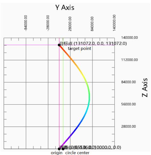
Action decomposition: the two axes of XOY plane do plane are action, and the arc track is determined by the starting point, center, target coordinates and path selection on the selected plane. The Z-axis moves in a straight line at a uniform speed, and the moving distance is the difference between the starting point of the Z-axis and the target point. The three axes start and stop at the same time, and the three-axis speed is decomposed into XOY plane linear speed and Z-axis linear speed.
