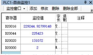
The given position (D20016) and the current position (D20044) are constantly changing. The current given speed (D20020) is the speed 131072 set in the command, and the current axis state (D20000) is 2, indicating that the axis is in the motion state with the termination speed of 0.
