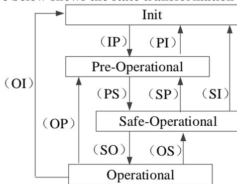
※The (IP) etc. in the state transformation diagram is the abbreviation of state transformation
