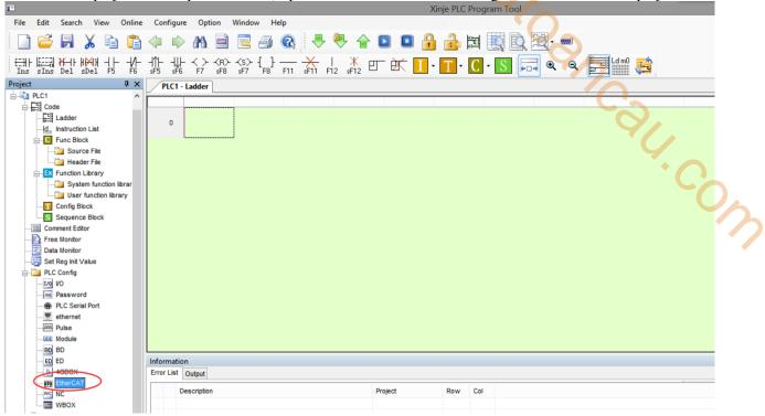
The EtherCAT parameter configuration interface is divided into master station configuration area, slave station display area and slave station configuration area.
