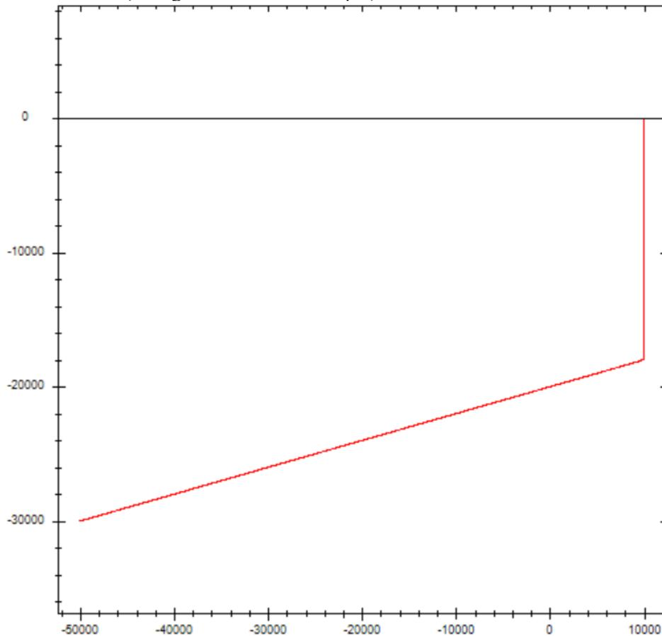
In the figure, the abscissa is X axis and the ordinate is Y axis. Coordinate starting point (- 50000, - 30000), after G\_PTP motion, the X and Y axes move to the target position (10000,0) at their respective default speeds.
