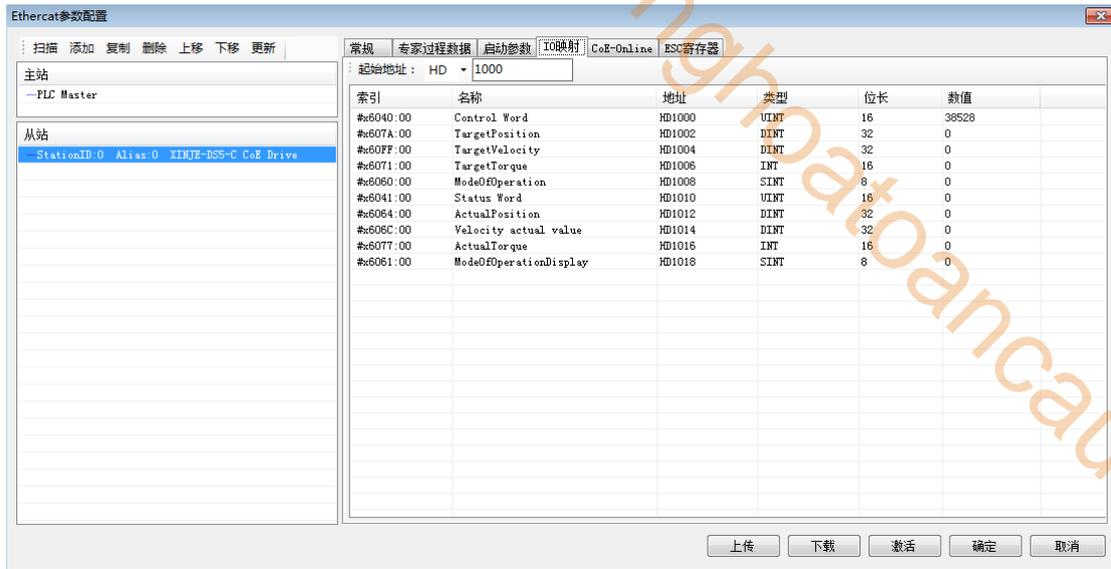
The allocated RxPDO and TxPDO will be mapped to the register starting from the [start address], and the register types can be HD and D. Modifying the [start address] will automatically arrange the addresses according to the parameter order. If there is a duplicate address with other stations, an error will be reported and the address will be automatically arranged to a non duplicate address.
