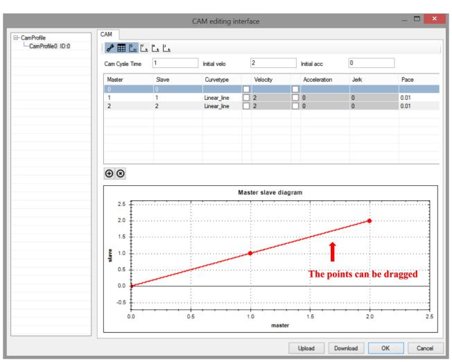
[main axis]: The point position of the main axis can be changed manually by double clicking. The subsequent point position must be greater than the previous point position. The number of main axis points cannot exceed 65535. The number of main axis points = (main axis final point position – main axis starting point position) / pace [slave axis]: The point position of the slave axis can be changed manually by double clicking.
