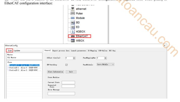
(2) confirm the PDO in the [expert process data] (The default configuration can meet the use of instructions. If necessary, other relevant parameters can be added).
