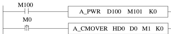
Since the current position of the motor is 4000, the [target position] parameter in the command should be 10000-4000 = 6000. The specific command parameter configuration is as follows:
