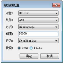
Configure two triggers, the object of which are all HD1012, the condition is AND, the mode is rising edge, the threshold value is 50000 and the other is 100000, the action is StopDisplay, enable is True.
