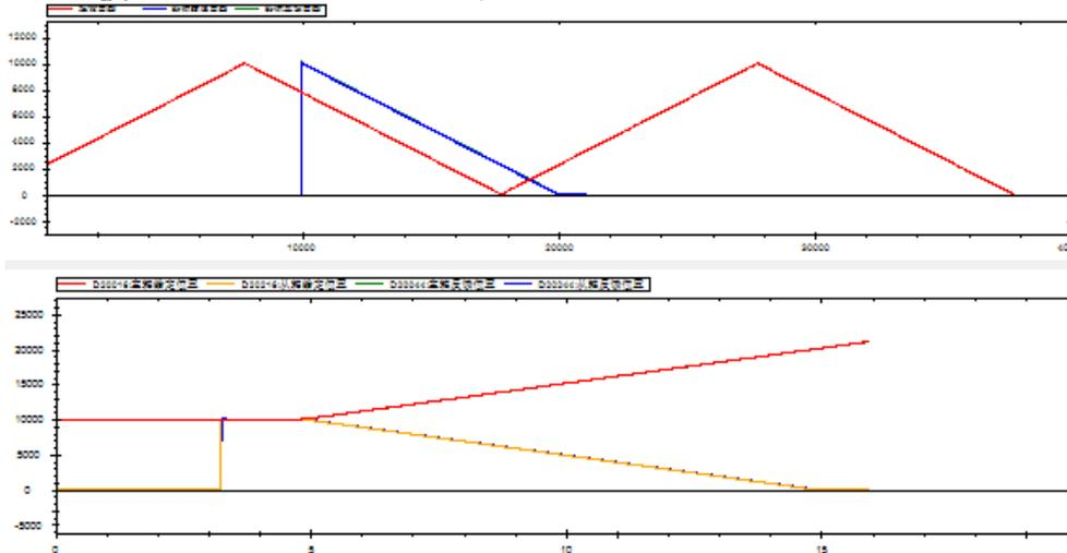
It can be seen that the slave axis position steps from 0 to 10000, the starting point of the track is (10000,10000), the cam table starting from main axis position 10000 is executed.
