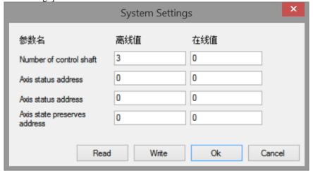
[number of control shaft]: it is SFD810, refer to chapter 5-1-3 (the offline value is the setting value in [the number of axes shown], the online value is the actual value in current register).
