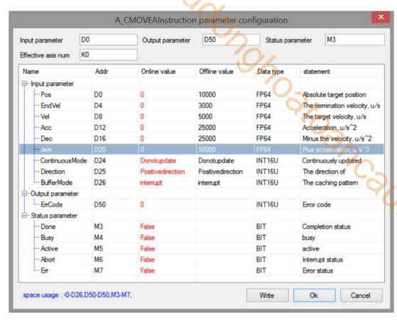
Note: To enable the axis through A\_PWR instruction. After confirming that the enabling is successful, turn M2 from off  $\rightarrow$  on and trigger A\_CMOVEA command, which runs to the target absolute position at the set speed, and then runs continuously at the termination speed. During operation, the state machine D20000+200\*N of the axis is 3.
