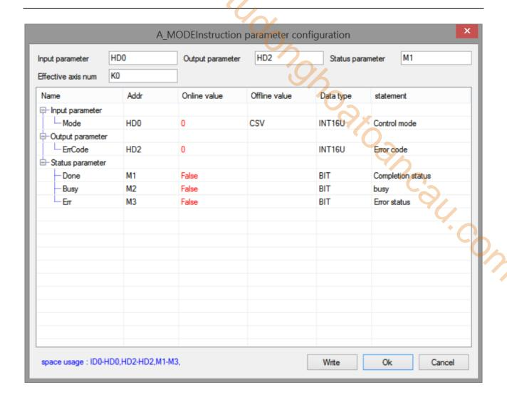
Note: if the command is executed successfully, the flag bit M1 changes to on, and the control mode of the specified axis will change to CSV mode (the value of 6060h is set to 9. See 4-3-5 control mode setting for control mode setting details).
