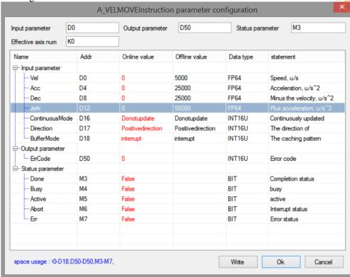
Note: To enable the axis through A\_ PWR command. After confirming that the enabling is successful, turn M2 from off  $\rightarrow$  on and trigger A\_VELMOVE command, which performs acceleration/deceleration with the set parameters, and then runs continuously at the target speed. During operation, the state machine D20000+200\*N of the axis is 3.
