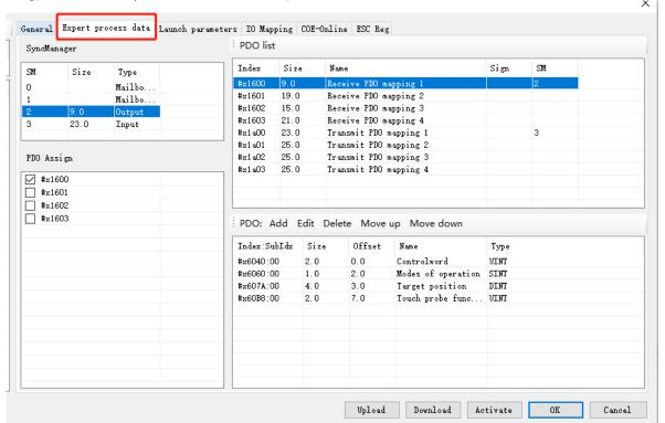
3 confirm the value of 6060h is 8 in [launch parameters]. 6060h value 8 represents the slave station is CSP mode.
