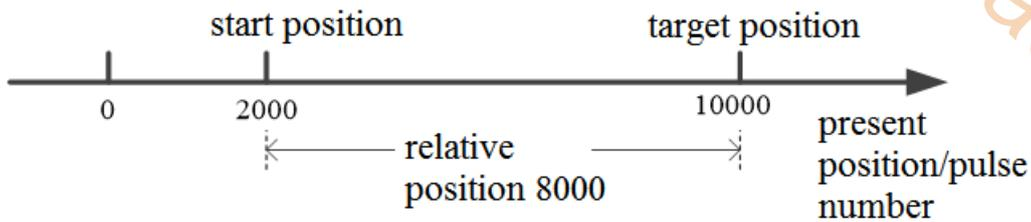
At the current position 2000, 8000 pulses need to be sent to run to the 10000 pulses position in the relative position mode. Similarly, 10000 pulses need to be sent to run to the 20000 pulses position.
