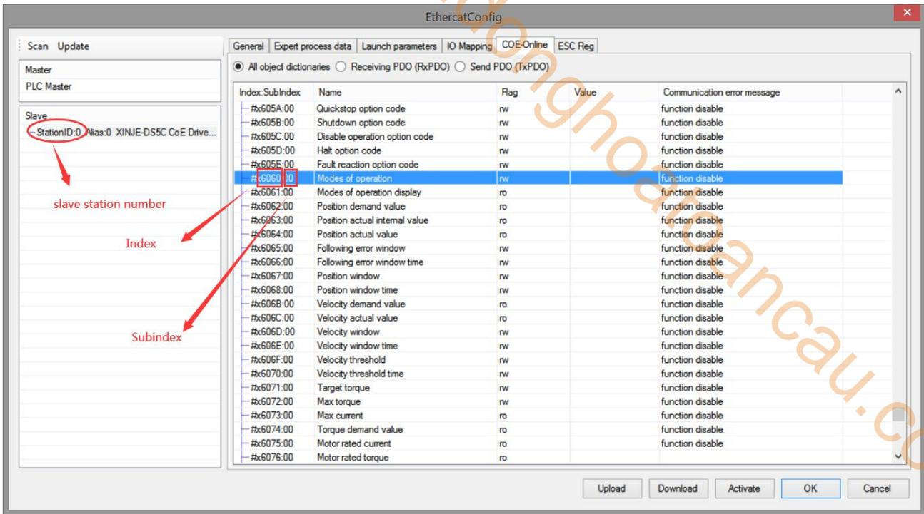
The figure shows the slave and the corresponding object dictionary index, read the value in slave object dictionary 0x6060: 00 of StationID0 to D0.
