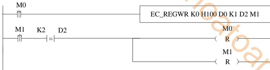
After operand S5 (M1) is set ON, check the status of S4 (D2). According to the status code, if the instruction is processed successfully, the read register can be set value. Since the completion mark M1 will not reset actively, it needs to be reset manually, so RST M1.
