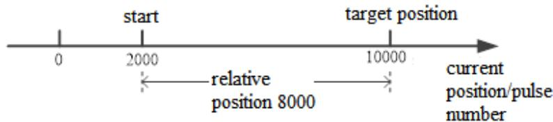
The present position is 2000, it needs to send 8000 pulses to move to 10000 pulses position in relative mode.
