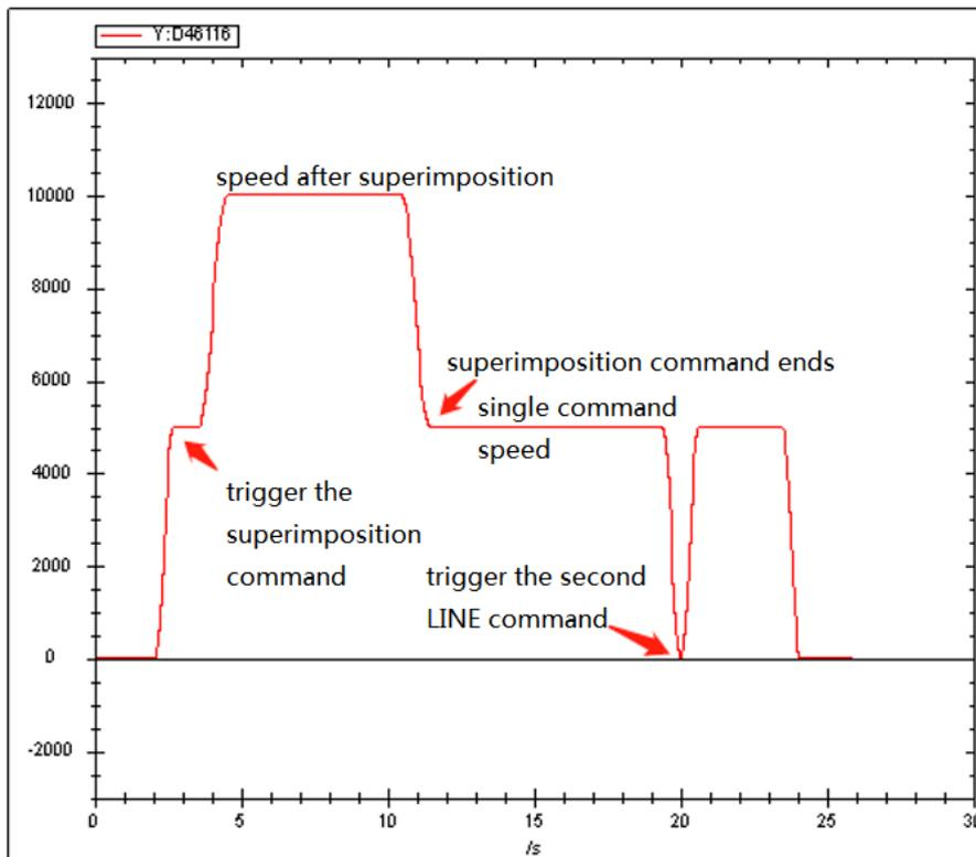
It can be seen from the speed curve that when the superposition instruction is executed, the speed will be superimposed on the basis of the original speed. After the execution of the superposition instruction, the previous speed will continue to execute until the execution of the instruction ends and the speed decreases to 0.
