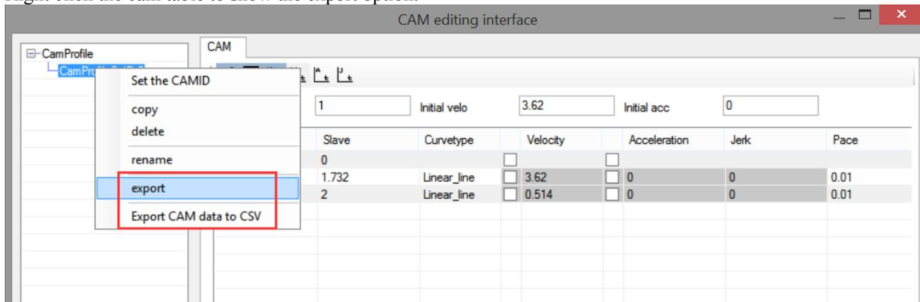
[export]: The cam table is exported. The generated file can be imported again in the cam table editing interface. The generated file is only a description file and does not contain the points in the cam table.
