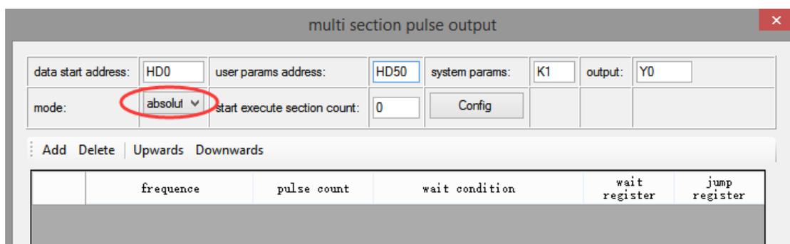
After choosing the mode, click the "Add" button in the configuration interface to add two continuous pulse parameters of forward rotation; after configuring, click the "Write to PLC" button to write parameters into the PLC, as shown in the following figure:
