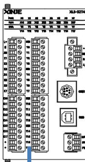
**Transistor output (Y0, Y1, Y2, Y3)**
