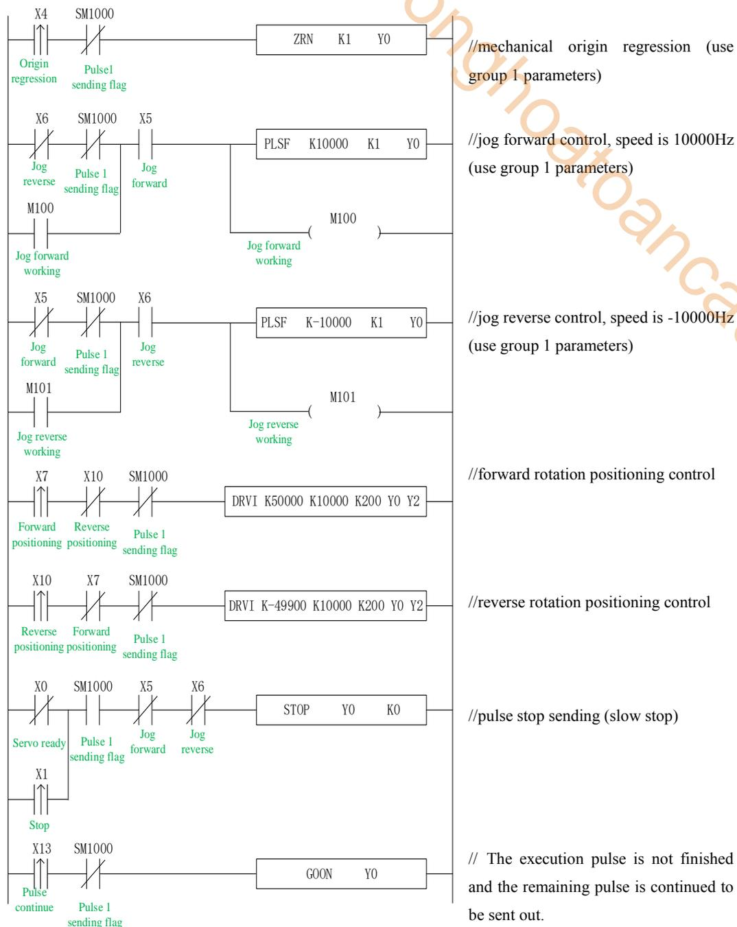
In the sample program, except DRVI and DRVA, all the system parameters used in the pulse instructions are group 1 parameters. So, we click "pulse configuration parameters" in the PLC programming software, as follows:
