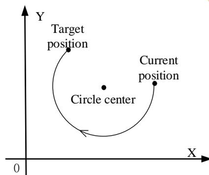
From the above figure, we can see that when we need to draw a whole circle, we only need to set the target position to the current position. CW has three modes. The usage of CW is described below.
