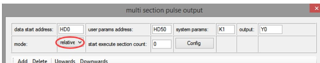
After choosing the mode, click the "Add" button in the configuration interface to add two continuous pulse parameters of forward rotation; after configuring, click the "Write to PLC" button to write parameters into the PLC, as shown in the following figure:
