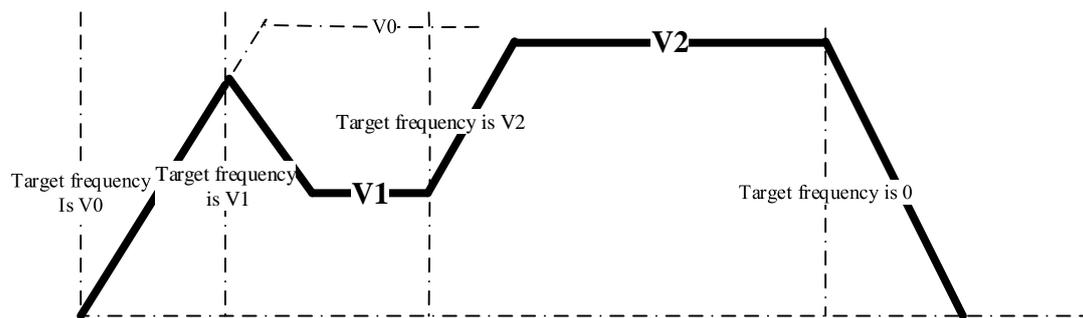
User set target frequency V1 ( $V1 < V0$ ,  $V1 < \text{present frequency}$ ) before reaching setting frequency V0, at this time, it will go to new setting frequency V1 as the down slope.
