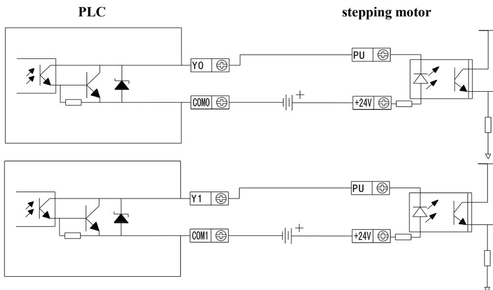
Note: If the pulse and direction terminals of the stepper motor are driven by DC5V, please connect 2.2K  $\Omega$  resistance behind the pulse and direction terminals.
