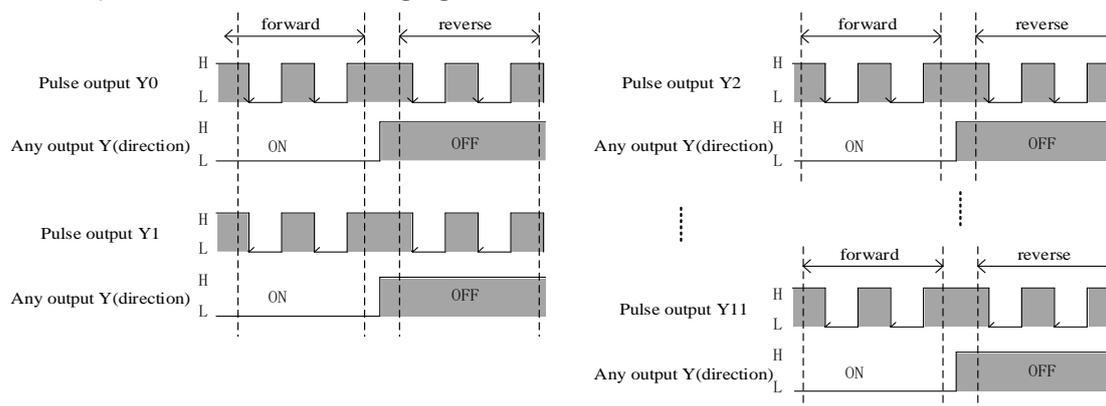
Note: ON and OFF represent the output state of the programmable controller; H and L represent the waveform of HIGH and LOW.
