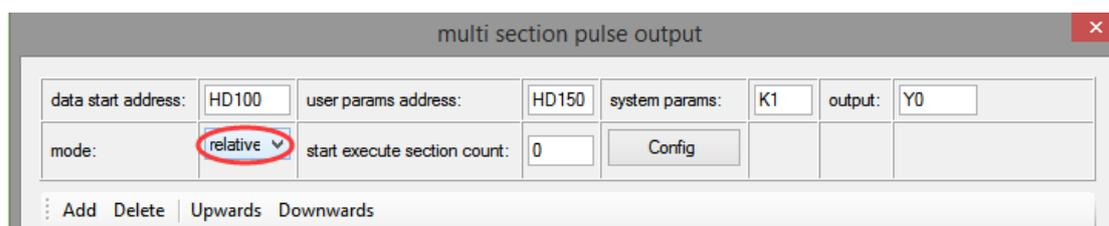
After choosing the mode, click the "Add" button in the configuration interface to add two continuous pulse parameters of reverse rotation; after configuring, click the "Write to PLC" button to write parameters into the PLC, as shown in the following figure:
