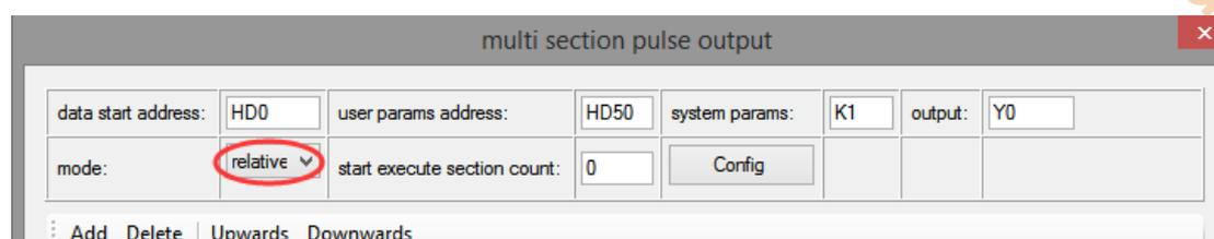
After choosing the mode, click the "Add" button in the configuration interface to add two continuous pulse parameters of forward rotation; after configuring, click the "Write to PLC" button to write parameters into the PLC, as shown in the following figure:
