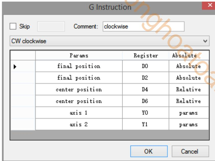
In the register list, double click the value can change the register address and axis output terminal. In the absolute list, double click the value can set the mode (relative/absolute). Double click the parameters can set the direction, speed, acc/dec time of the two axes, please see the follows:
