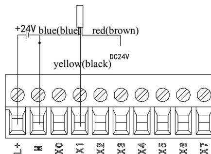
Three-wire (NPN) proximity switch wiring
