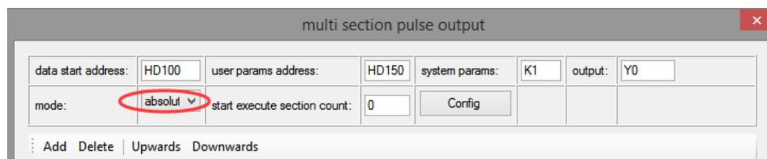
After choosing the mode, click the "Add" button in the configuration interface to add two continuous pulse parameters of forward rotation; after configuring, click the "Write to PLC" button to write parameters into the PLC, as shown in the following figure:
