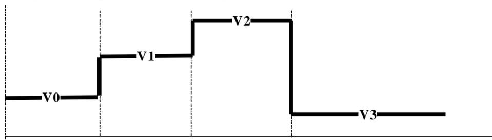
(B) Pulse default speed acceleration deceleration time is not 0
