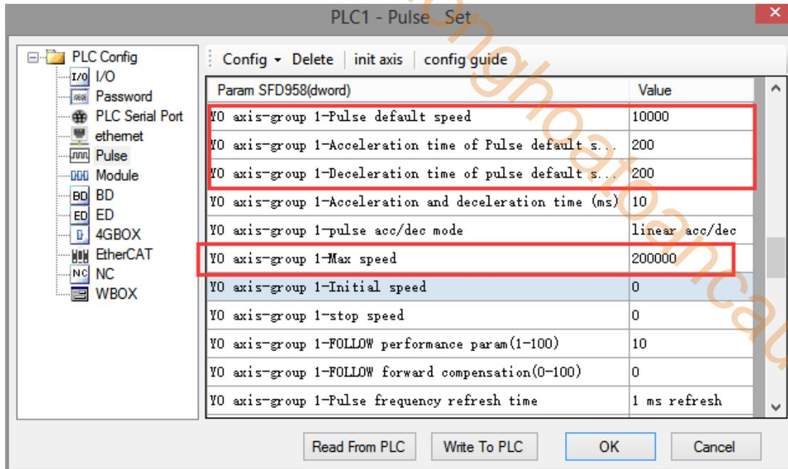
After configuring the parameters, click the "Write to PLC" button to write the parameters into the PLC. After downloading the program, power off the PLC and then power on again.
