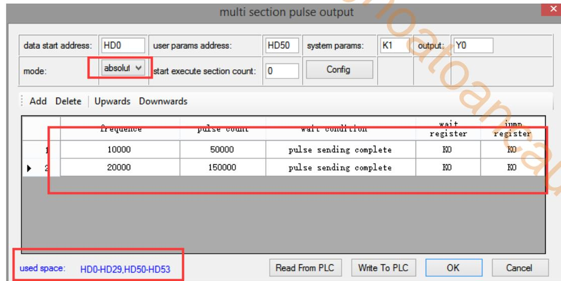
**Note:** Please note the range of real-time occupied registers displayed by "used space". Because the range of starting address of pulse parameter data of PLSR pulse instruction is HD0-HD29, and the range of system parameter block address is HD50-HD53, the range of real-time occupied registers address is not beyond the range. If the range exceeds, the error of pulse output will occur.
