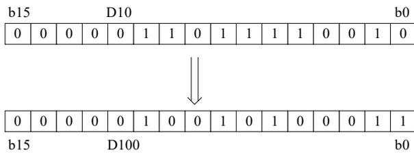
From the left second bit of D10, XOR each bit with the value after decoding, as the bit value after decoding (the left bit will not change). The transformation value will be stored in D100.
