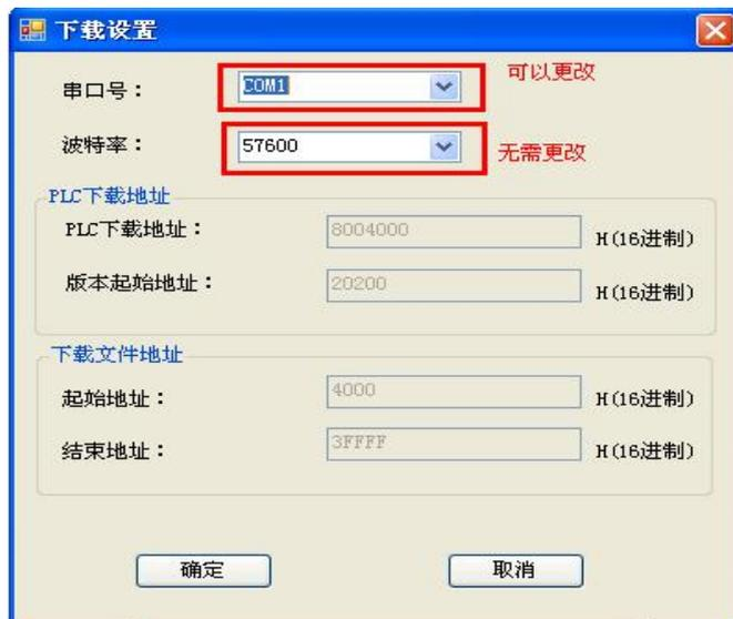
Note: set the com port, the baud rate is default setting, no need to change.
