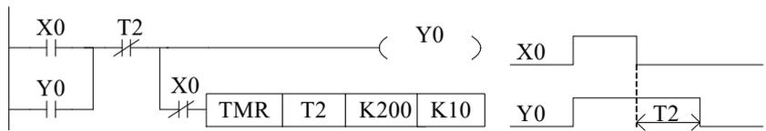
X0 is ON, output Y0. X0 changes from ON to OFF, delay 2s then cut off Y0.
