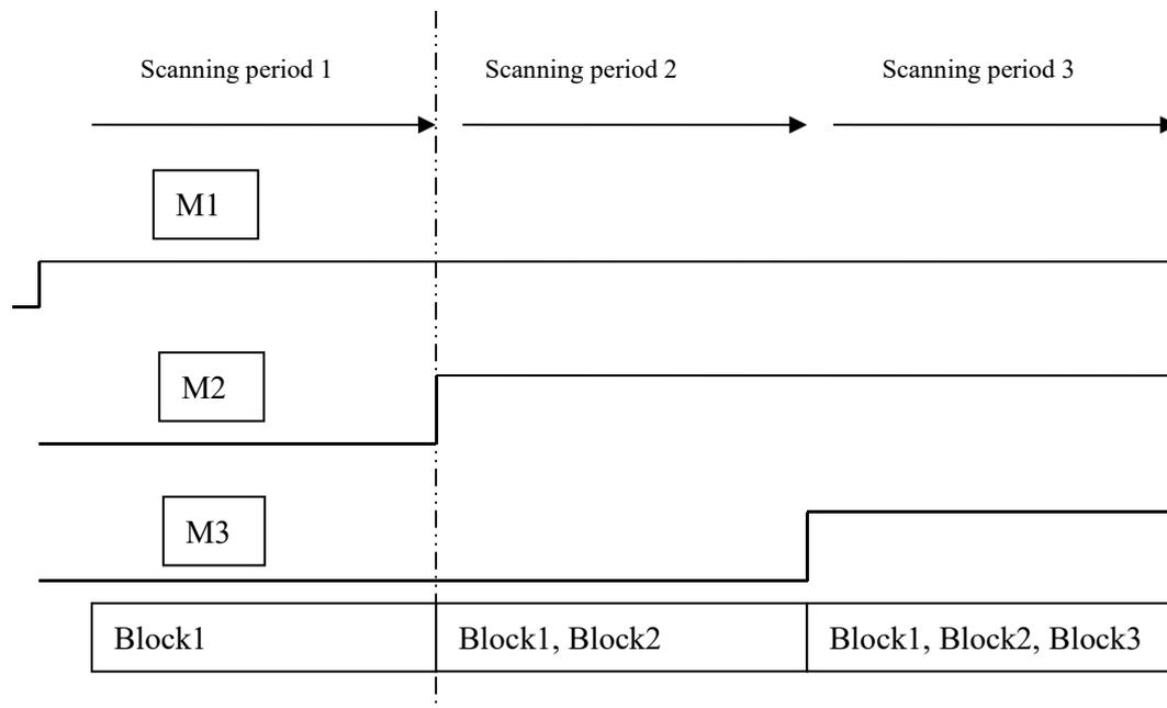
Note: When the program in the BLOCK is not executed and the triggering condition M is disconnected, the BLOCK will not stop immediately, but will complete the last scan, and will stop after the rest of the program has been executed.
