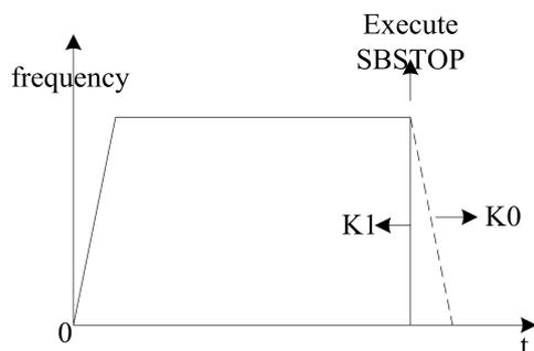
K2: Destructive slow stop BLOCK, that is, when the pulse is being sent, the SBSTOP condition holds, then the pulse will slow down along the slope, without to use with the SBGOON instruction, so the remaining instructions will not be executed. After executing this instruction, the BLOCK can be restarted. (Note: K2 mode is only supported by V3.4.2 and above PLC)
