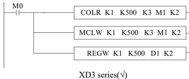
Note: XD/XL series PLC sequence block has cancelled Modbus communication instructions, which is replaced by the current Modbus instruction handling mode.
