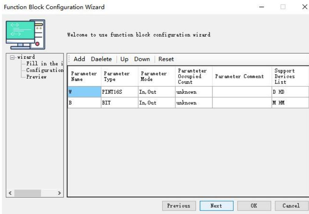
After completing the parameter configuration, click "next" to display the preview interface of the source file. If there is a problem, click "previous" to reset the parameters. If there is no problem, click "OK" to complete the addition of the source file.
