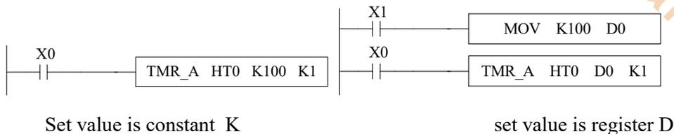
(2) Time unit is 10ms, set time is K10, the real time is  $10\text{ms} * 10 = 0.1\text{s}$
