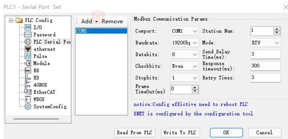
**Port No.:** It refers to Port of PLC, COM0 refers to Port 0 (RS232), COM1 refers to Port 1 (RS232), COM2 refers to Port 2 (RS485) or Port 2-RS232 (RS485) or Port 2-RS485 (RS485), COM3 refers to Port 3 (left extended ED port), COM4 refers to Port 4 (upper extended BD port 1), COM5 refers to Port 5 (upper extended BD port 2).
