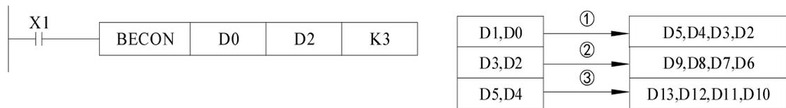
Note: The register header address of a double - precision floating-point must be even.
