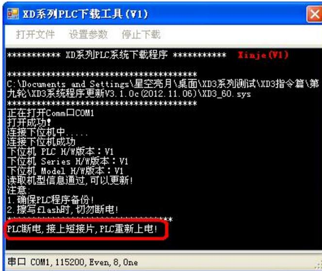
Cut off the power of PLC, connect the short jumper, then power on the PLC again.
