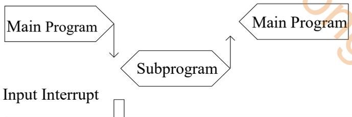
**Note: The external interruption of XC series PLC cannot be activated by rising edge and falling edge at the same time; but XD/XL series PLC supports rising edge and falling edge activation meantime.**
