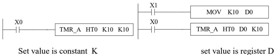
(3) Time unit is 100ms, set time is K1, the real time is  $100\text{ms} * 1 = 0.1\text{s}$
