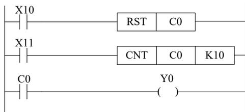
C0 increase counts the X11 OFF to ON times. When C0 reaches K10, C0 will become OFF to ON. When X11 becomes OFF to ON, the C0 current value will keep increasing, and the C0 coil will still be ON. When X10 is ON, reset the C0 coil.
