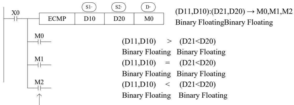
When X0 is OFF, even ECMP doesn't run, M0~M2 will keep the status before X0 is OFF.
