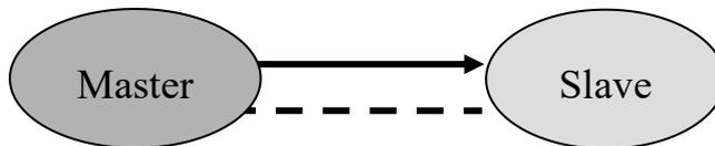
There is dotted line in the diagram. It means any PLC can be master station when all PLC in the network don't send data. As the PLC do not have unified clock standard, communication will fail when more than one PLC send data at one time. It is not recommended to use.
