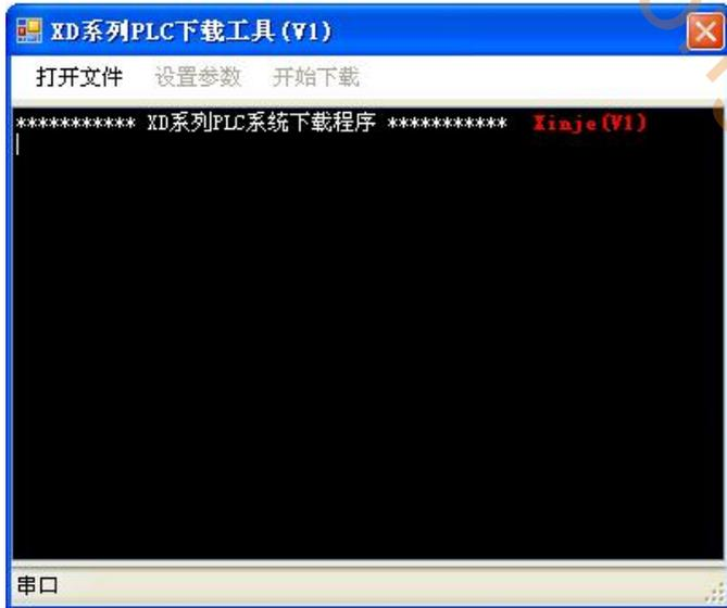
Click "Open File", choose the PLC model for updating. (Note: XD3\_16.sys fit for PLC model XD3-16, XD3\_60.sys fit for PLC model XD3-32 and XD3-60):
