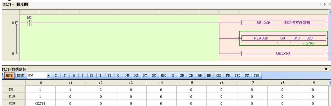
In the above figure, the SD card reading instruction is: READSD D0 D10 D20, and the function meanings of each parameter are as follows:
