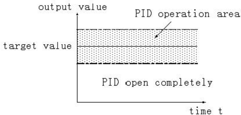
If the target value is 100, PID operation zone is 10, and then the real PID's operation zone is from 90~110.
