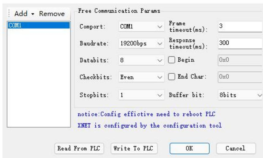
**Port No.:** It refers to Port of PLC, COM0 refers to Port 0 (RS232), COM1 refers to Port 1 (RS232), COM2 refers to Port 2 (RS485) or Port 2-RS232 (RS485) or Port 2-RS485 (RS485), COM3 refers to Port 3 (left extended ED port), COM4 refers to Port 4 (upper extended BD port 1), COM5 refers to Port 5 (upper extended BD port 2).
