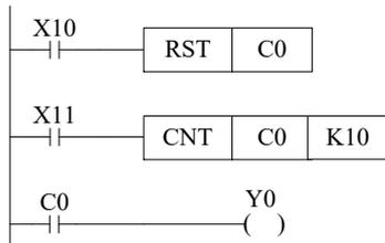
The counter C0 increases one when the X11 drives once. When C0 value reaches 10, the output acts. Then X11 drives again, C0 will continue increase one. If X10 is ON, the C0 and output will be reset. The counter set value can be constant K or register. For example, if D10 is 123, the set value is equal to K123.
