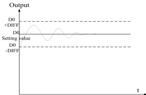
To enter the auto tune mode, please set bit7 of (S3+ 2) to be 1 and turn on PID working condition. If bit8 of (S3+ 2) turn to 1, it means the auto tune is successful.
