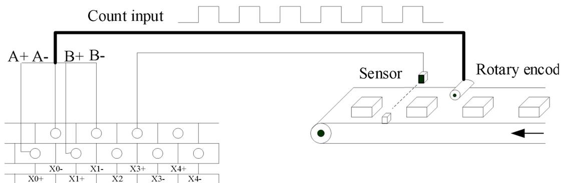
(3) When the counting frequency is higher than 25Hz, please select a high-speed counter.
