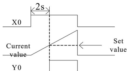
If X0 is ON, then T0 accumulates 10ms pulse based on the current value; when the accumulation value reaches the set value K200, the timer output activates. I.e. the output activates 2s later. If X0 is OFF, the timer resets, the output resets;
