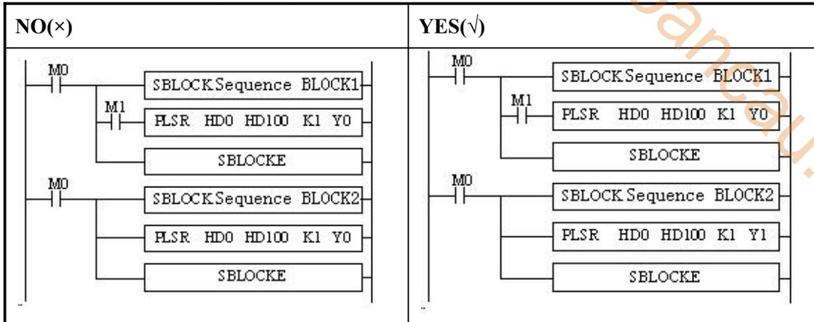
(2) Do not use the same pulse output terminal in BLOCK and main program.
