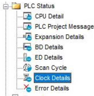
Then click write into the current time.the PC will auto-write the current time to the PLC.
