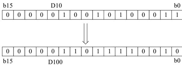
Each bit of D10 will XOR with the bit on its left side. As the related gray code, the left bit will not change (the left bit is 0); the transformation result is stored in D100.
