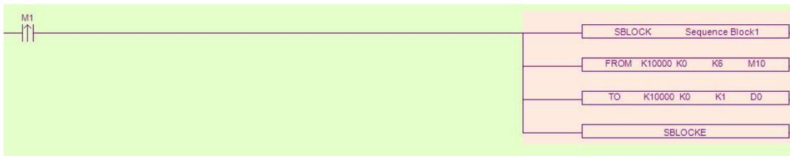
Note: As shown in the figure above, in V3.4 and above version software, when the module number is set to K0~K15, the corresponding ladder diagram will be displayed as K10000~K10015.
