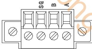
Please use twisted pair cable for RS485. (See below diagram). But shielded twisted pair cable is better and the single-ended connects to the ground.
