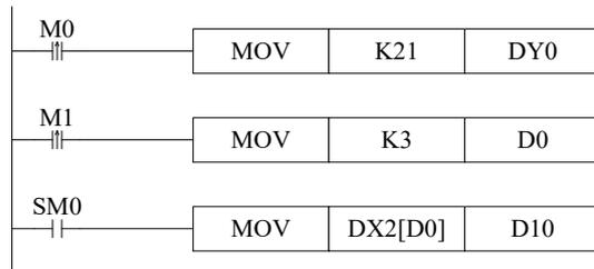
When M0 changes from OFF to ON, the value in the word which is combined by Y0~Y17 equals to 21, i.e. Y0, Y2, Y4 become ON.
