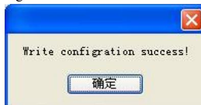
(7) Close XINJEConfig tool, cut the PLC power and power on again to make the settings effective.
