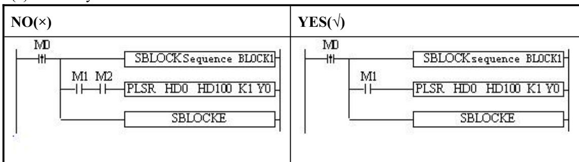
(4)The SKIP condition only can use M, X, can not use other coil or register.
