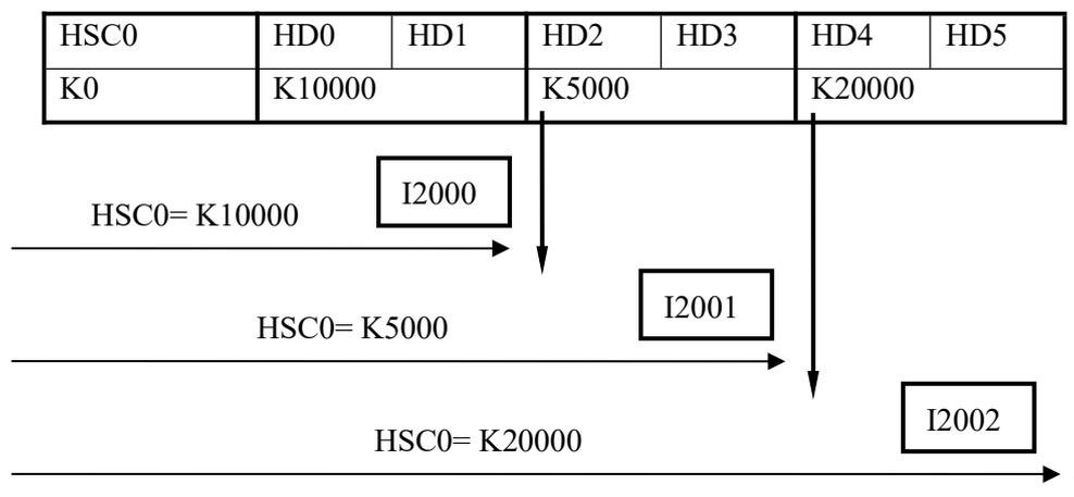
Note: When absolute counting is performed in non-cam mode, counting interrupts are generated sequentially, i.e., segment 1 interruption, segment 2 interruption, segment 3 interruption... When a segment interrupt occurs, no interrupt occurs even if the count value reaches the set value of the segment again.
