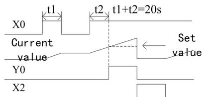
If X0 is ON, HT0 accumulates the 10ms pulse based on the current value. When the accumulation value reaches the set value K2000, the timer output activates.
