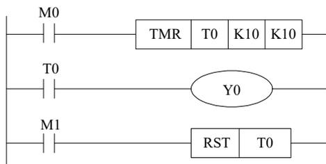
When M0 is ON, T0 starts to timing. When T0 reaches K10, T0 coil is ON. Then T0 continues timing. When M1 is ON, reset the T0.
