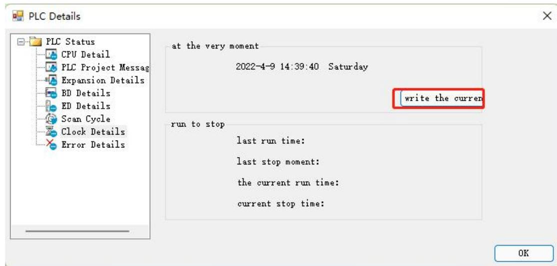
Then click write into the current time.the PC will auto-write the current time to the PLC.
