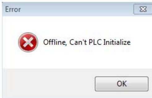
In both cases, use PLC system update tool to update PLC system, and PLC and PC will be connected successfully if system is updated (For more steps about system update, please refer to Q3 related content).
