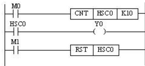
Increase count the OFF to ON times of M0. When the count value reaches set value (value of K or D), the count coil will be ON. When M1 is ON, the count coil of HSC0 reset, the current value becomes 0.
