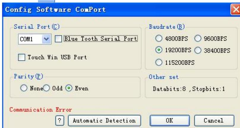
Choose correct communication serial port according to your PC actual serial port.; baud rate selects 19200BPS, parity check selects even parity, 8 data bits, 1 stop bit; you can also click 'check' button directly in the window, and communication parameters will be selected by PLC itself. 'Connect to PLC succeed' will be displayed on the left bottom of window as below:
