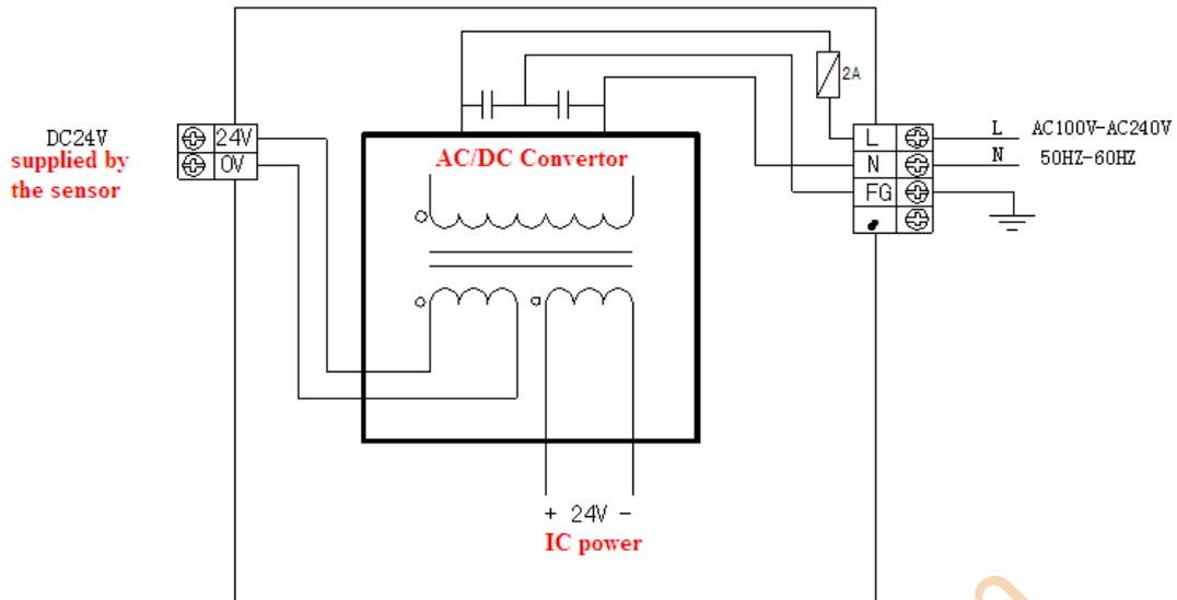
※1: Connect the power supply to L, N terminals.
