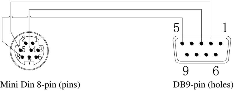
Note: above diagram is for DVP cable. If it is XVP cable, please connect pin1 of Mini Din8 and pin7 of DB9 based on above diagram.
